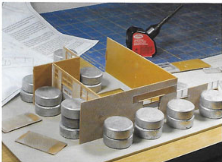
Above: The round puck-like disks are weights that I used to hold the plastic walls in place to allow the glue to dry. These weights are among the handy helpers I keep around for building hobby projects such as this railroad station kit.
